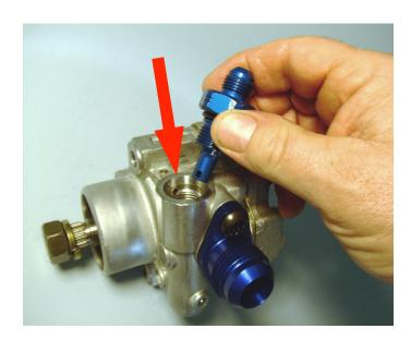
If the piston stays stuck down in the bore, the pump cannot create any output pressure and the power steering will not work.
