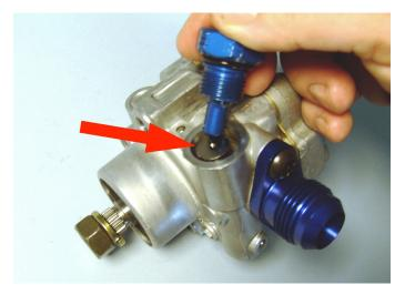
Normal: the piston will pop out as the fitting is removed.
