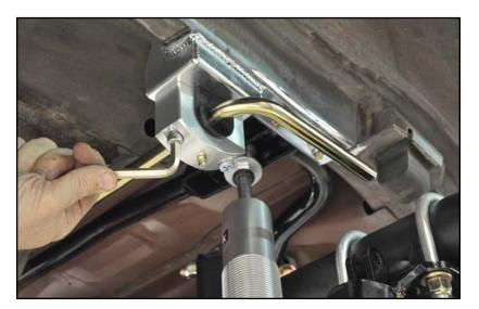
8. Measure from each billet housing to the outside of the bar on each side to verify that the anti-roll bar is centered.
