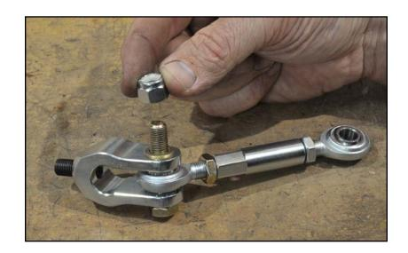
15. There are three detents in the anti-roll bar. we are going to tuse the softest set to strart, this is the one at the end of the bar. Slide each clevis over the end of the anti-roll bar until the set screw lines up with the last detent. Tighten the set screw and then the locknut. This is the initial installation position for the anti-roll bar.
