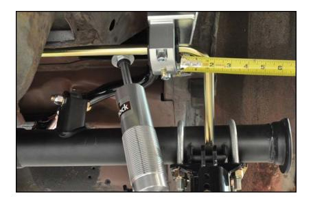
9. It is a good idea to chase the threads in the adjuster before assembling it. Use a 3/8-24 tap to do this. The end with the hex is left hand thread
