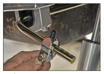
16. Bolt the opposite end of each adjuster endlink assembly to the tabs on the lower axle brackets, using 3/8-24 x 1-3/4" hex bolts, aircraft washers and locknuts.
