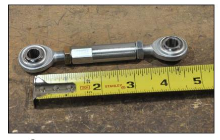
12. Use a 3/8-24 tap to chase the threads in the clevis.
