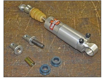
2. Press two bushings into each shock eye.
