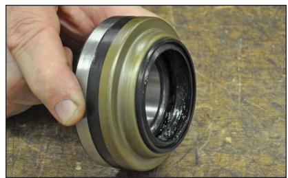
21. Slide the axle bearing assembly over the axle shaft with the seal facing toward the axle flange.
