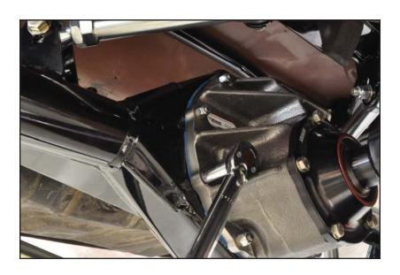
INSTALL TIP: Any studs that have not held their threaded position can be identified by comparing the thread engagement with the nut. To tighten the stud without removing the third member, remove the locknut and thread two 3/8-24 jam nuts onto the stud. Jam the two nuts together and tighten the stud by turning the bottom nut in the counterclockwise direction.
