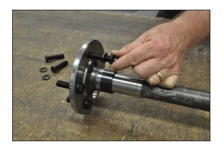
13. Apply red Loctite® 271 to the 1/2" length of exposed threads, and then hand tighten the studs until seated against the flange.
