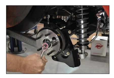
42. As a final step, the third member can now be filled with gear oil through the filler cap on the back of the housing. It will take approximately two quarts to fill to the correct level. The plug in the side of the third-member case must be removed during filling. The case is full when the fluid level has reached the height of the plug.
