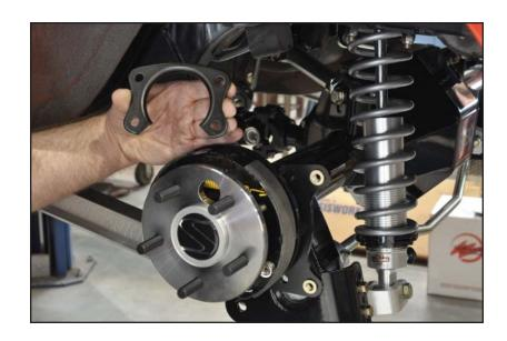
41. Stock-style T-bolts are inserted from the back side of the housing end and the nuts tightened through the access hole in the axle flange.
