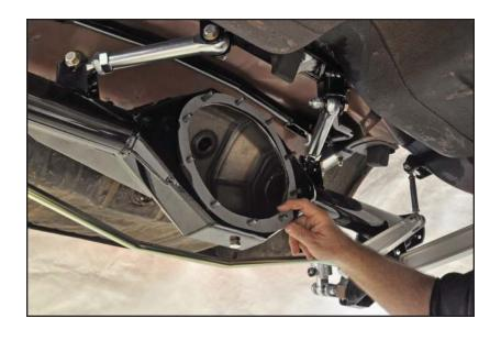
33. Carefully place the third member over the studs. Due to the weight of the third member it may be difficult to slide fully into position. A rubber mallet can be used to carefully walk the third member into position.
