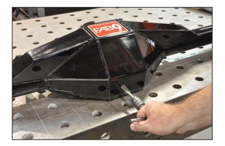
2. Slide the copper seal over the magnetic drain plug and thread it into the housing. Tighten to 40 lb-ft.
