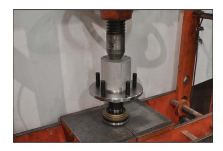
23. Apply pressure to the bearing assembly until it is completely seated against the bearing stop on the axle.
