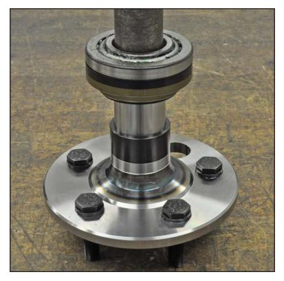
22. Set the axle and bearing into a hydraulic press as shown. Make sure the V-blocks are tight around the axle, so you are only putting pressure on the center bearing collar not on the outer race.
