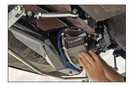
34. Slide the 3/8" aircraft washers over the studs and then the locknuts. The nuts on the two lower studs will need to be tightened with a wrench.
