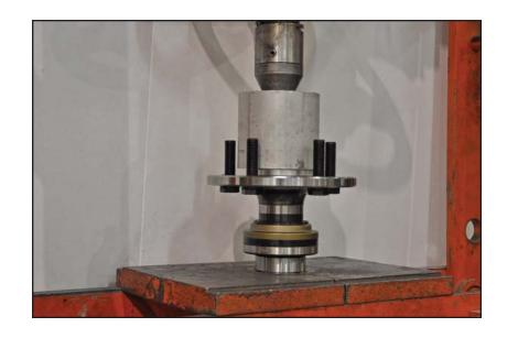
28. The axle bearing installation is complete and the axle ready to install into the housing once the third member is in place.
