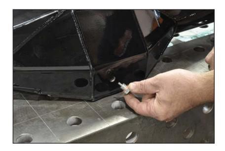
3. Use a 3/8-24 NF tap to chase the threaded holes on the face of the housing before installing the studs.
