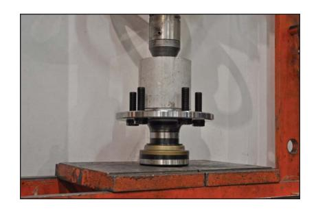
24. An additional ring referred to as the "wedding ring" is included with the axle bearing and must be pressed on after the bearing.
