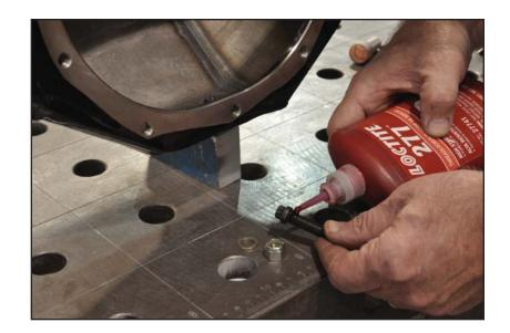
5. Thread the 12-point bolts into the holes in the face of the housing from the inside. Tighten the bolts to 35 lb-ft. Let the Loctite® cure for 24 hours before installing the 3rd member.
