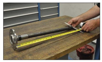
11. Measure the distance from the far side of the axle flange to the bearing stop and verify against the packing list.
