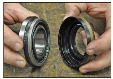
20. Once the seal is installed the bearing is ready to be pressed onto the axle.
