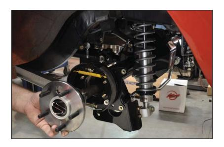
40. The axle bearing retainer sits against the axle seal and share mounting hardware with the disc-brake-caliper mounting bracket.
