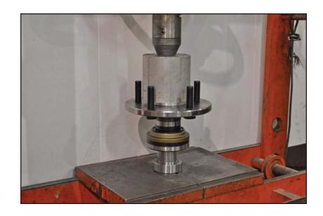
27. The fit of the wedding ring is much tighter and will take more pressure to fully seat compared to the axle bearing.
