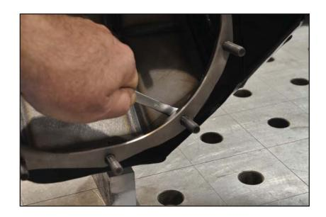
6. Thoroughly clean the inside of the housing and axle tubes, using a clean shop rag. A board or broom handle can be used to push the rag through the axle tubes.
