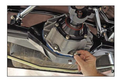
35. Hand tighten all of the locknuts. Once they are all seated, final tighten the locknuts to 35 lb-ft.
