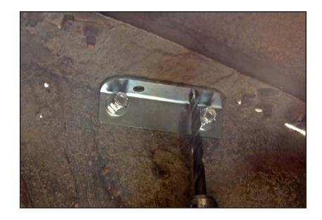
12. Install 3/8" button head bolt, two flat washers, and locknut. Tighten to 30 lb-ft.
