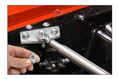
20. Tighten the fasteners to 40 lb-ft.
