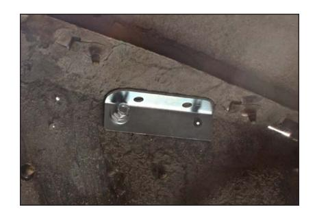
7. Drill the second hole through the inner fender. Make sure the bracket is square to the top of the inner fender.
