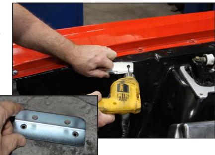
4. Using a 3/8" bit, drill one of the two holes needed to mount the bracket.
