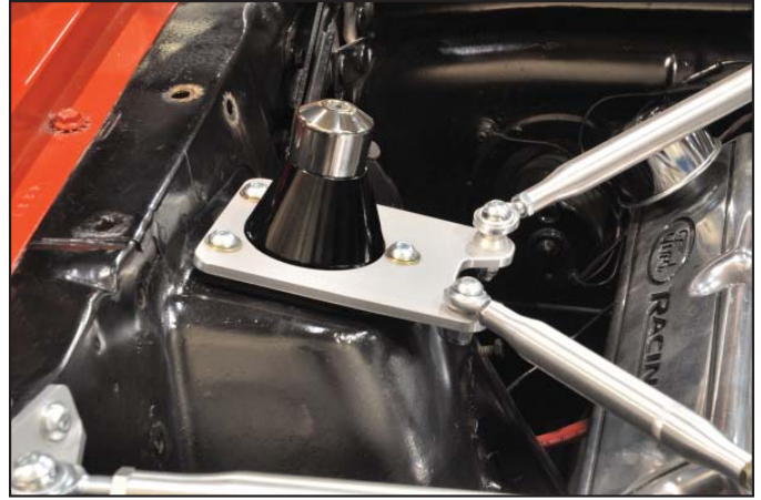
Bolt-On Coil-Over mounted BELOW - standard ride height
