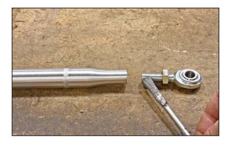
19. Bolt the radius-rod assembly to the first fender bracket using a 1/2-13 x 1-3/4" button-head bolt, and locknut.
