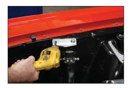
8. Install the second set of 3/8" mounting hardware and tighten to 30 lb-ft.
