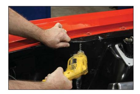
5. Bolt the aluminum fender bracket and steel support bracket to the inner fender using a 3/8" button-head bolts, two flat washers, and a locknut.
