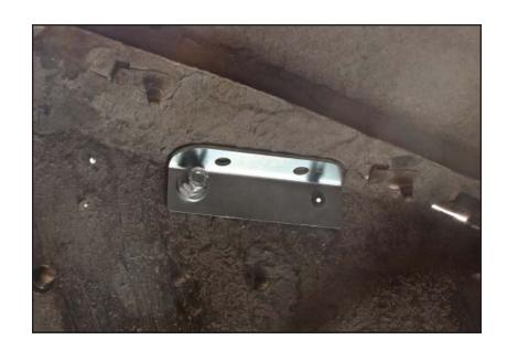
7. Drill the second hole through the inner fender. Make sure the bracket is square to the top of the inner fender.
