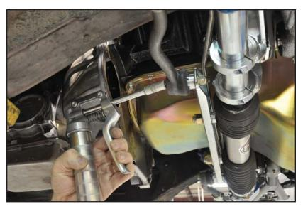
20. Once you have the front end aligned tighten the jam nuts against the adjuster.
