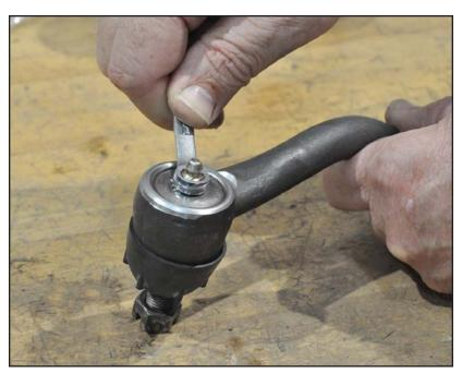
11. Insert the tapered adapter into the end hole of the rack's center link or factory drag link.
