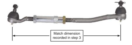
10. Install the grease zerk fitting into the tie rod ends and tighten.
