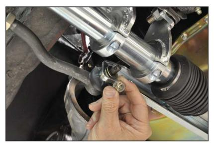
14. Tighten the locknut with a 5/8" wrench. You will have to push the tie rod into the tapered adapter while tightening the locknut.
