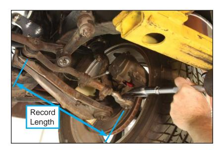
4. Apply anti-sieze or similar thread lubricant to internal threads at each end of the adjusting sleeve.
