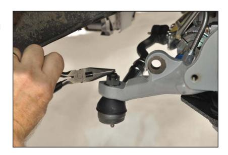
19. Grease the tie-rod ends with a common grease gun until the boot starts to bulge.
