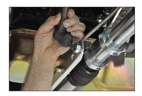
13. Place a 7/16" hardened flat washer over the tie rod stud, followed by a 7/16" locknut.
