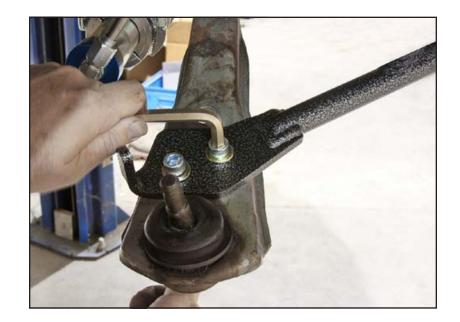
22. Using the pivot stud hex, adjust the length of strut rod to position lower control arm square to frame rail.
