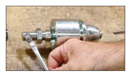
12. Screw pivot assembly into strut rod.
