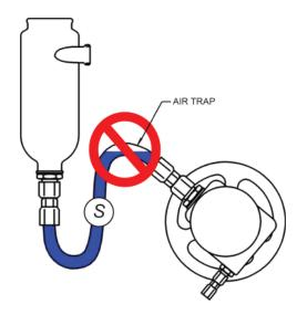
Verify that all fittings and hose ends are tight and that the area around each connection is completely dry before filling the system with fluid. If the lines must be removed use two wrenches to remove the hose end without unscrewing the fitting.
