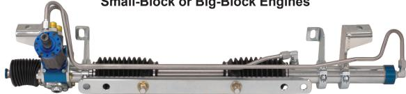
Description: High-clearance power TCP Rack & Pinion with mounting brackets and hardware ONLY. Bracket and center-link combination increases oil-pan and exhaust header clearance. This product requires installation of bump steer kit (TCP TIER-XX) to maintain correct steering geometry.
