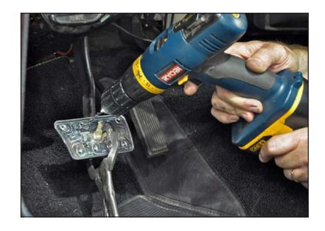
9. Clamp the gas pedal pad in place and use the same procedure as the brake pedal to install.
