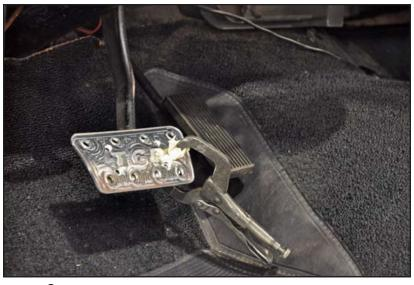
3. Using the pedal pad as a jig, drill the first hole with a 3/16" (.187") drill bit.
