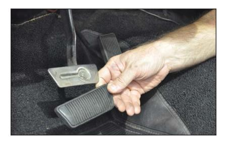
Position billet brake pedal pad over the factory pedal and secure into place using a C-clamp or vise-grip pliers. Use masking tape to protect the pedal cover from being scratched.
