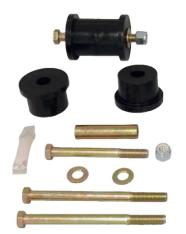
**Description:** Polyurethane bushing set, includes bushings, sleeves, mounting hardware, and poly lube. Fits 2"-bore x 2-1/2"-wide front leaf-spring eye with 1/2" mounting bolt. Directly replaces RB82 rubber bushing.
