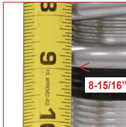
Measure the bottom end of the spring.
