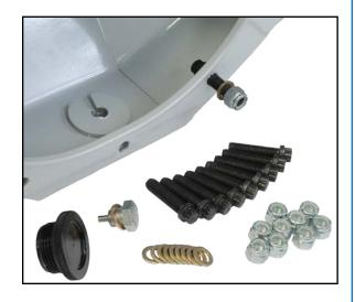
the axle tube. Equalized pressure improves the effectiveness of all seals and gaskets for trouble free extended use. If an external fluid catch can is required, axle vents can be easily removed using the 7/16" hex and replaced with an appropriate 1/8" NPT fitting. Third-member mounting hardware consists of high-strength 12-point studs, hardened SAE flat washers, and nylon insert locknuts.
